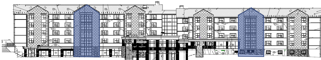
Figure 33: Bathroom Stack Location | AE211
