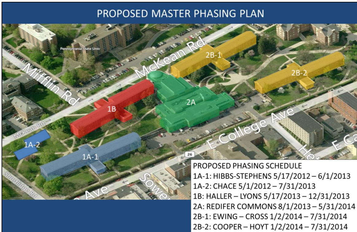
Figure 70: Proposed Phasing Plan
